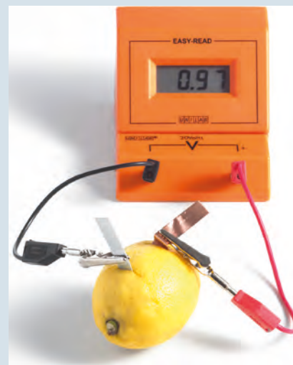
FIGURE 9.2.3 An electrical cell made from a lemon
