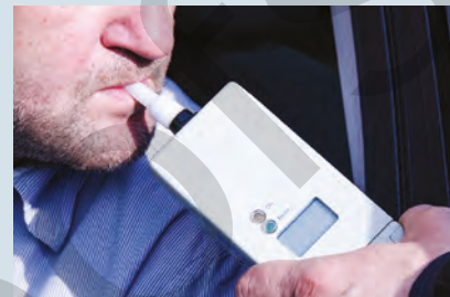
FIGURE 9.4.12 Hand-held breathalysers are a type of fuel cell.
