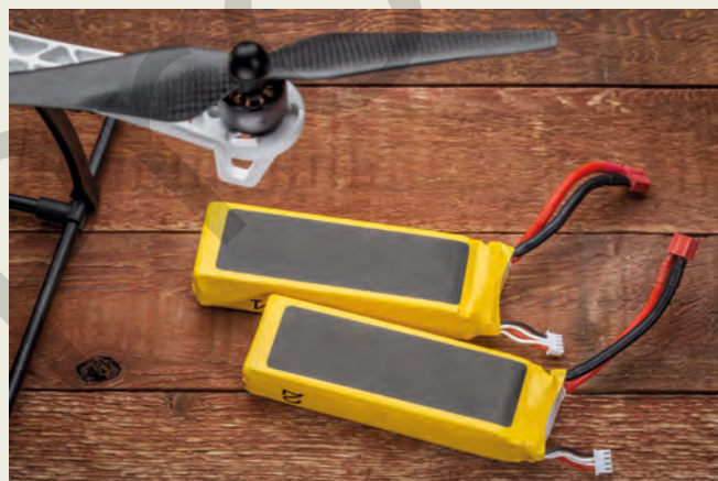
FIGURE 9.4.8 Lithium-ion power supplies are used in drones and radio-controlled models.
