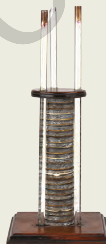
FIGURE 9.1.2 An original voltaic pile. The pile is 15 cm high and contains alternating copper and zinc discs separated by cardboard.
