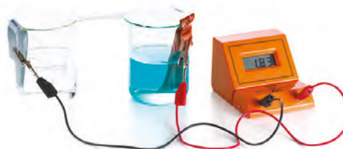
FIGURE 9.1.3 Construction of a galvanic cell from simple laboratory equipment.
