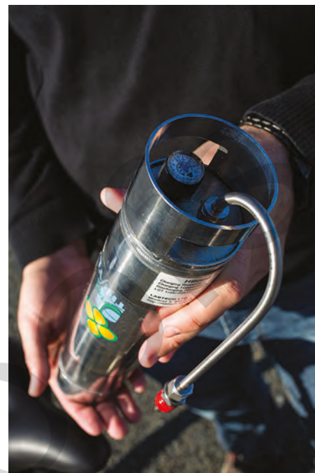
FIGURE 9.4.9 A hydrogen fuel cell for an electric bicycle. The hydrogen bicycle operates like a standard electric bicycle, but the battery lasts three times longer.
